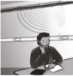
Fig. R15 Power cables and metallic busways magnetic field radiations
